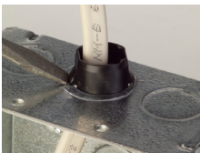
Easy Removal - Push the wing tab of the connector with a screwdriver. Push the connector through the knockout towards the inside of the box.
